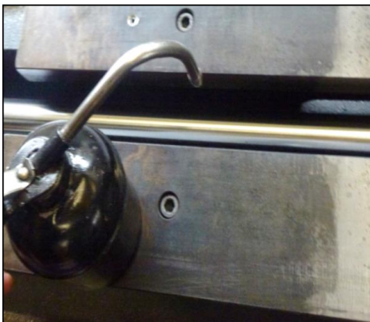
1.6) Lubricate the vice clamping shaft.
