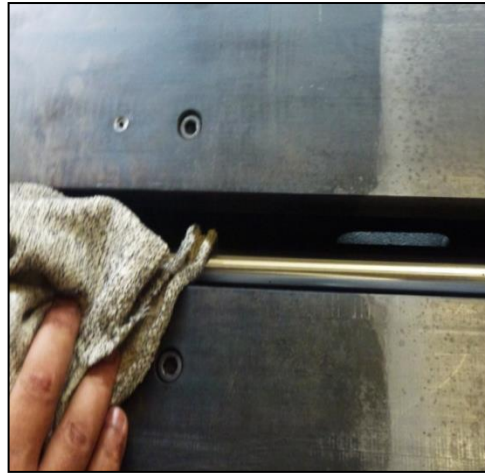
1.5) Clean the vice clamping shaft.
