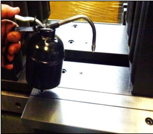
1.4) Lubricate the upper clamping blocks.
